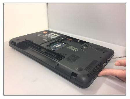
Use a metal spudger and run it along the edges of the computer to take off the plastic back cover.
