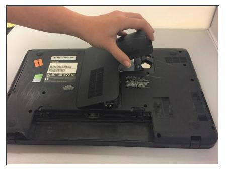
• Remove the middle plastic cover to expose the hard drive.
