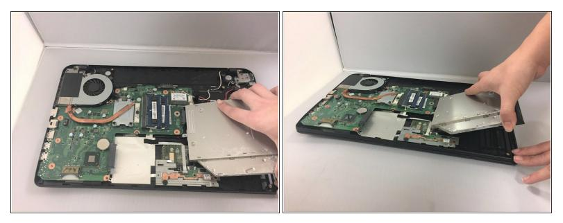
• Grab hold of the optical drive and elevate it slightly and remove it from the computer.
