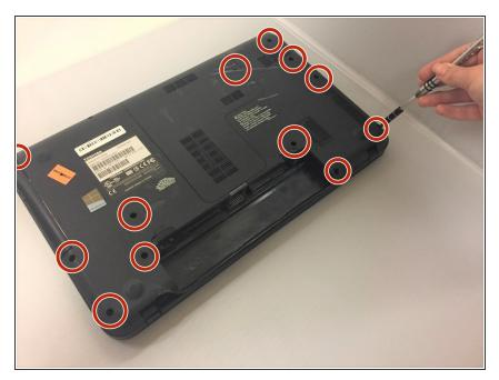
• Use the Phillips #1 screwdriver to unscrew the thirteen screws on the back of your device.
