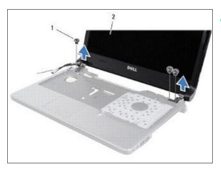
Use the alignment posts to place the NEW display assembly on the computer base.
