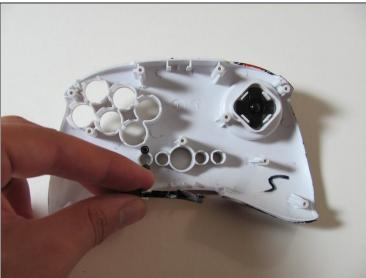
• Pull the plastic piece out from the bottom of the controller.
