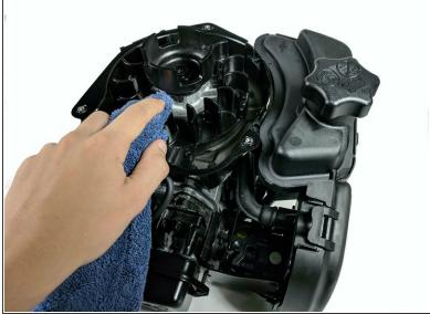
Using compressed air or a rag, clean debris from the flywheel.
