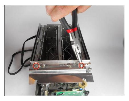
Remove the top panel by bending the tabs on each side straight up.
