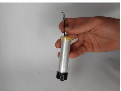
Remove the plunger from the device.
