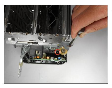
Remove the two 8mm screws on the bottom of the plunger using a Tripoint Y1 screwdriver.
