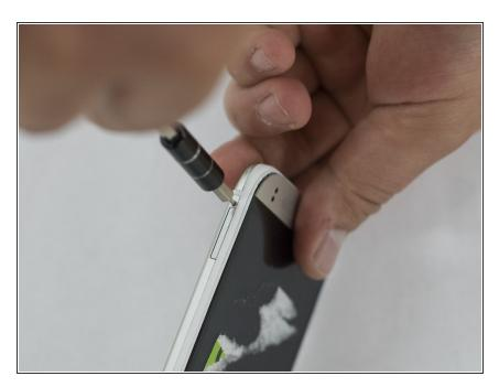
Use the sim eject tool to remove the SIM cards on either side of the phone.
