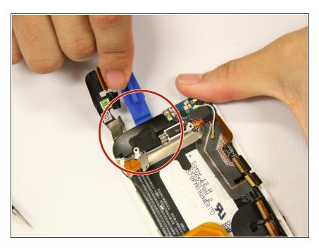
With a plastic opening tool, remove the black speaker at the bottom of the phone.
