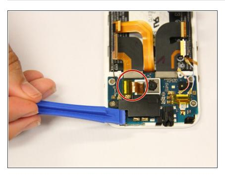
Remove the gold tape at the top right corner of the phone and disconnect the ribbon wire from the circuit board.
