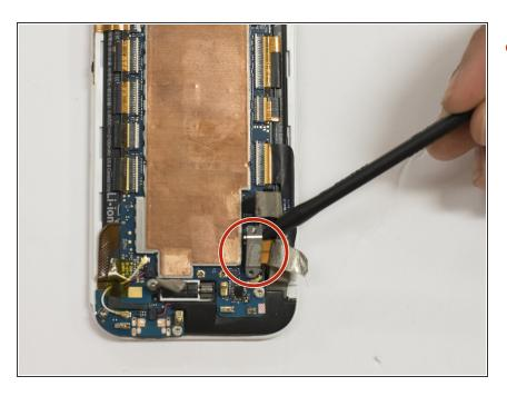
Remove the two 1 mm screws at the bottom right of the motherboard using a Torx 4 screwdriver.
