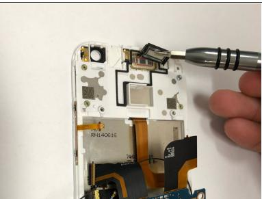
Using a plated screwdriver, remove the magnetic speaker from the phone itself.
