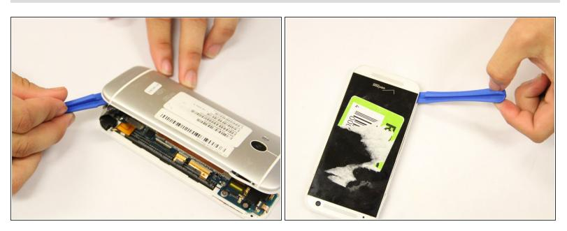
Use the plastic prying tool to pry off the back cover. Place the tool in the SIM card insert and lift off the back cover with force. Continue to do this all around the phone.
