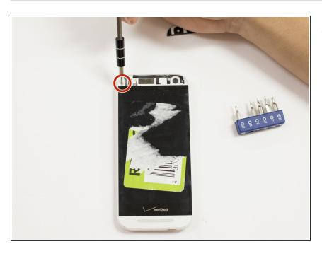
Remove the single 3 mm screw that is on the top left side using a Torx 4 screwdriver.
