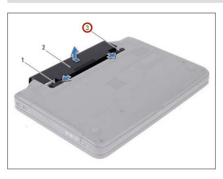
Slide the battery lock latch to the unlock position until it clicks into place.
