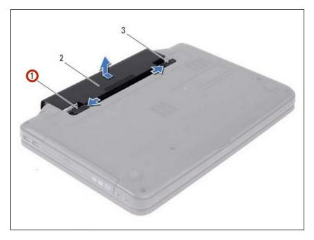
Slide and hold the battery release latch in the unlock position.
