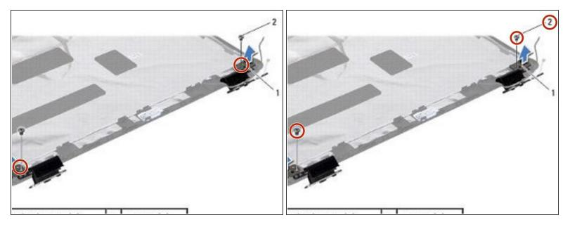
Align the screw hole on the display hinges with the screw hole on the display cover and replace the two screws (one on each side).
