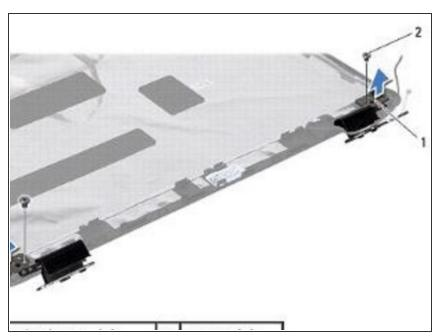
• Route the Mini-Card antenna cables on the **NEW** display hinge.
