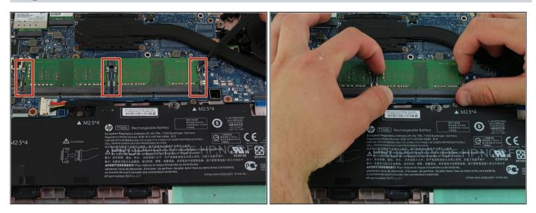
• Using your fingers, remove the clips on the sides of the sticks of RAM by pulling up and towards you.
