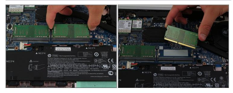
• Once the side gates are removed the stick of RAM will pop up and you can pull it out.
