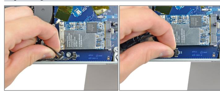
• Disconnect the HDD fan and power button from the logic board by pulling their connectors straight up off the sockets on the logic board.
