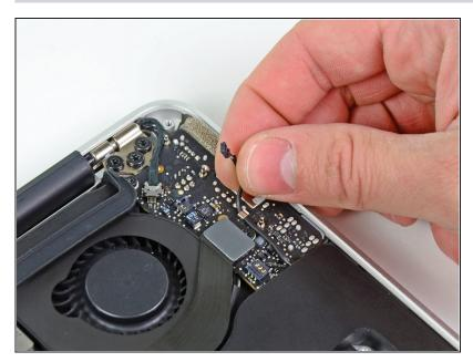
De-route the left speaker cable from its retaining clip on the I/O board.
