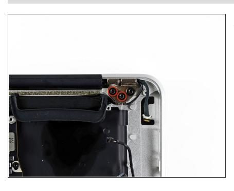
Remove the two 4.9 mm T8 Torx screws securing the antenna cable retainer on the left display hinge to the upper case.
