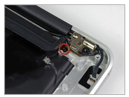
Push the antenna cable retainer out of the way and remove the 3 mm T5 Torx screw securing the end of the heat sink to the upper case.
