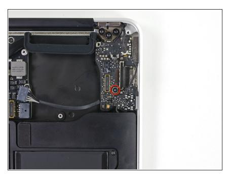
Remove the single 4.0 mm T5 Torx screw securing the I/O board to the upper case.
