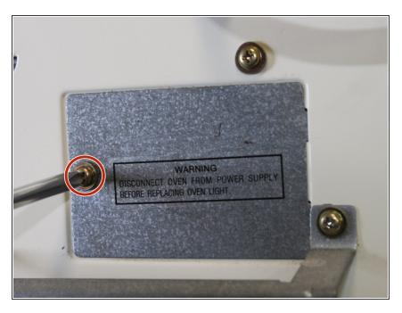
Unscrew the screw holding the metal panel in place.
