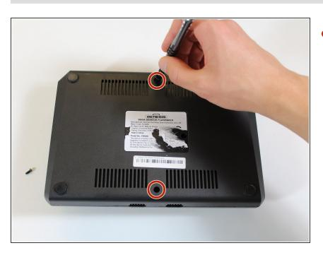
Remove the two visible screws on the bottom with the Phillips #000 screwdriver.
