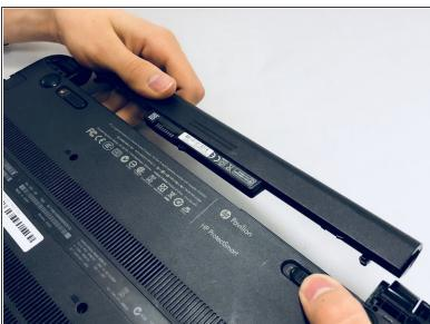
Carefully pull the battery away from the device.
