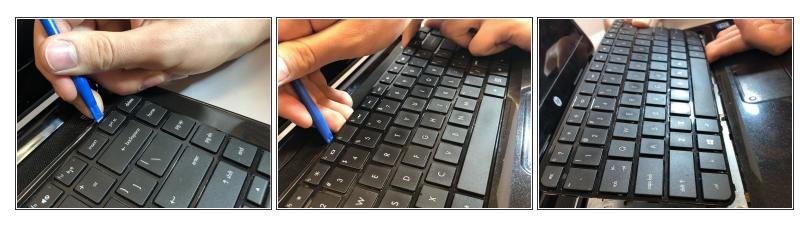
Using a plastic opening tool, pry up along the edge of the keyboard.
