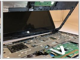
Disconnect the touch pad wire by flipping the black lever with a plastic spudger.
