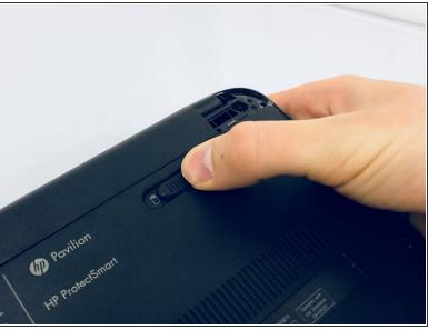
Press the switch on the right-hand side of the back of the device towards the center until the gray battery icon is no longer visible. This will eject the battery.
