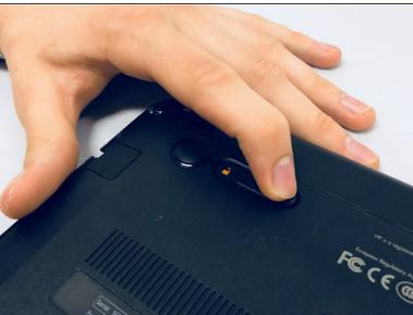
Flip the computer over and move the battery lock switch to the "unlocked" position (marked by an orange lock icon).
