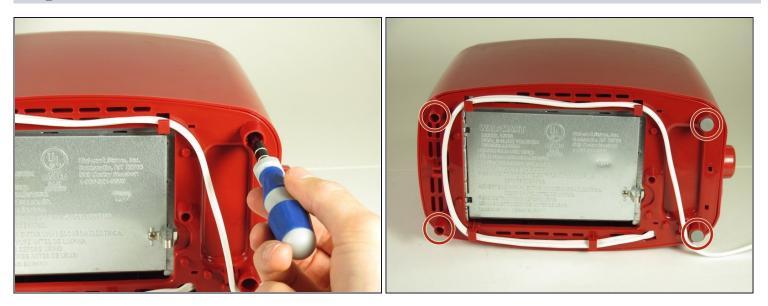
• Use a Phillips #2 screwdriver to remove four 12 mm screws at the base of the toaster shell.
