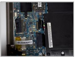
Using an iFixit opening tool and your other hand, gently lift the connector up from the tape wrapped around the connector wires and pry the connector from the motherboard.
