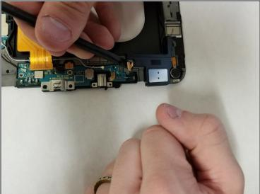
• Use the flat end of the **spudger** to snap the ribbon connector off of the motherboard.
