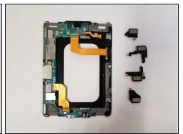
• Use the pointy end of the **spudger** to snap the speaker module off of the motherboard.
