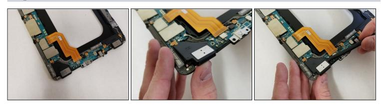
• Use your finger to snap one side of the speaker module off of the motherboard. Use the flat end of a **spudger** to snap off the other side.
