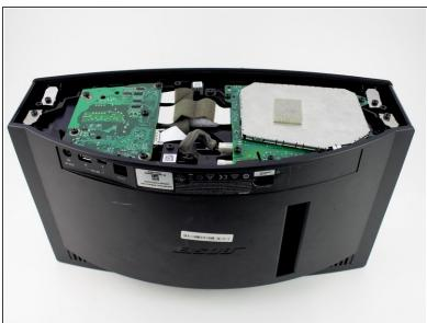
• Remove the four 15.5 mm PH2 screws securing the base plate to the device.
