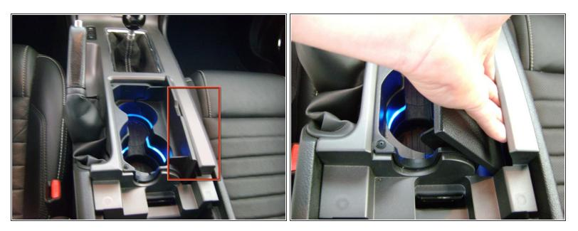
Grip the right side of the console and pull up towards the passenger seat to remove it.
