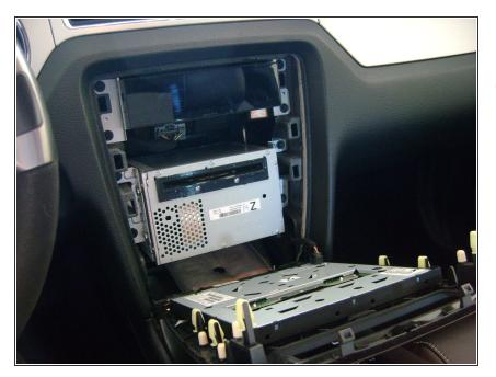
Inspect the interior of the center console for damaged wires or other faulty components.
