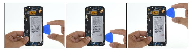
• Slide the pick along the edge to cut through the adhesive.
