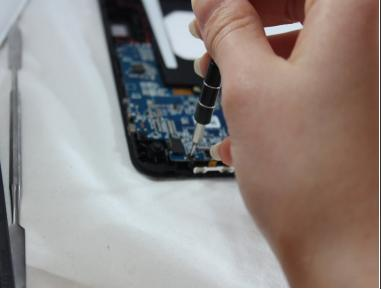
Use a Phillips #00 screwdriver to remove the five 2mm screws from the motherboard. There are two on the left edge and three on the bottom edge of the motherboard.
