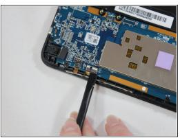
Using a spudger, disconnect the two ribbon cables on the top right and the three on the bottom left of the motherboard.
