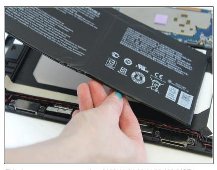
Remove the battery from the device.
