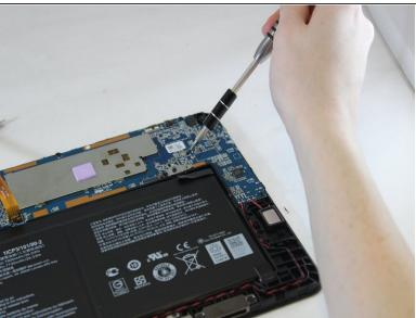
Using the Phillips #00 screwdriver, unscrew the two 2mm screws at the top right of the battery.
