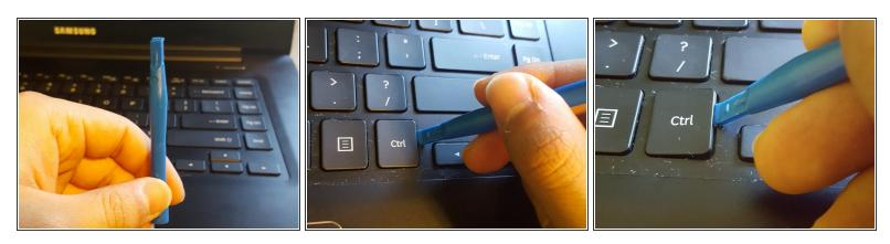
Insert a plastic opening tool underneath a key.
