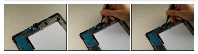
• Using the <u>tweezers</u>, remove the green protective film from the connector between the rear camera and the motherboard.
