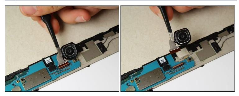
• Pull the connector out of the slot using tweezers and remove the camera.
