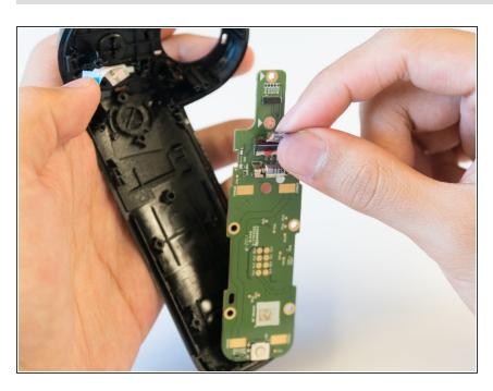
Pinch the orange ribbon cable and pull toward yourself to remove the motherboard.
