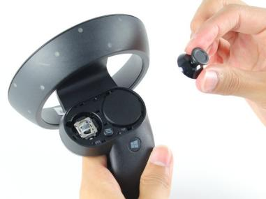
Grab the joystick and pull away from the controller to remove it.
