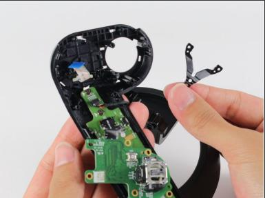
Insert your finger underneath the black plastic "V" and scoop up to remove it.
