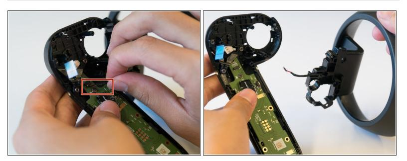
Grab the black and red wires attached to the motherboard and wiggle the connector out of the socket.
