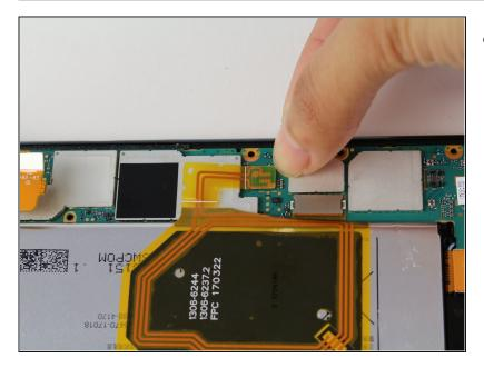
• Insert your nail under the center topmost connector and push to loosen it.
