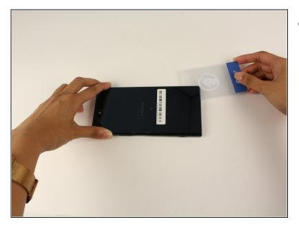
• Slide a thin <u>plastic card</u> under the back panel and around the perimeter of the phone to remove the adhesive.
