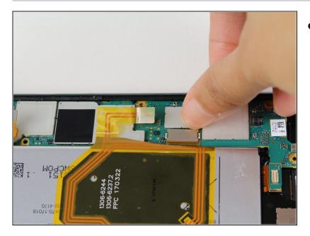
• Insert your nail under the metal tab of the connector above the battery and push to loosen it.
