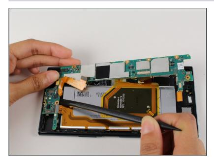
• Insert the spudger in the gap between the motherboard and the left side of the battery to further lift out the motherboard.
