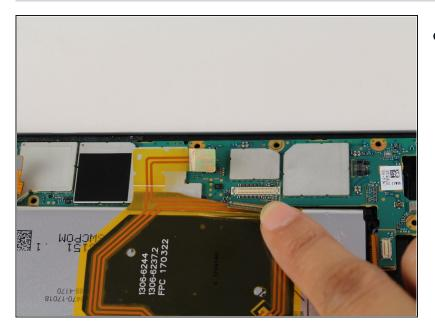
• Pull the metal tab of the connector towards you with your fingers to disconnect the pins.
