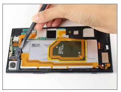
Place the spudger under the bottom left frame piece and lift to loosen it.
