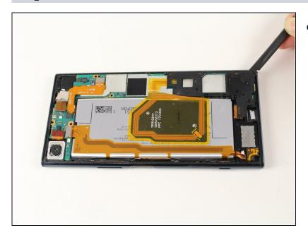
Place the spudger under the top right frame piece and lift to loosen it.
