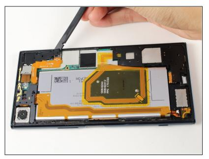
Place the spudger under the top left corner frame piece and lift to loosen.
