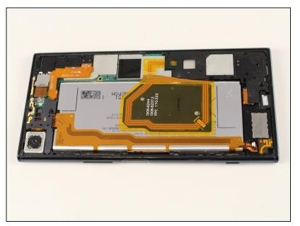
Orient the phone horizontally with the front screen facing down and the camera on the bottom left corner.
