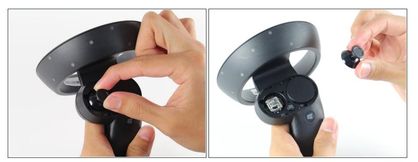
• Grab the joystick and pull away from the controller to remove it.
