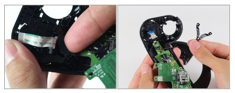
Insert your finger underneath the black plastic "V" and scoop up to remove it.
