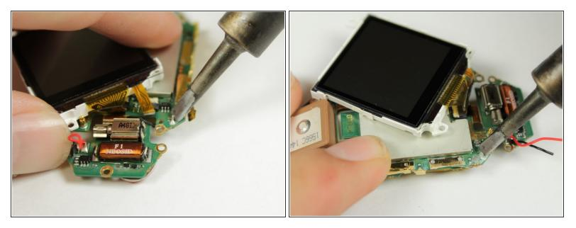
To remove the battery, desolder the black and red wires connecting the battery to the motherboard and remove the battery. See this guide on <u>How To Solder and Desolder Connections</u> for additional help.
