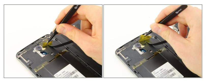
• Remove the yellow Kapton tape by using the tweezers to peel it up and away from the device.
