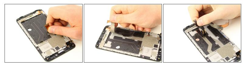
• Using your fingers peel up the LCD flex cables. These cables are black and flat.
