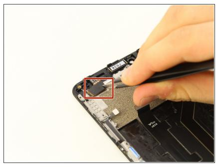
• Disconnect the digital flex cable connector, located at the top left of the phone, using a pair of tweezers.
