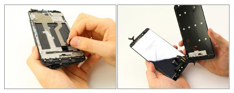
• Push the digitizer flex cable through the hole in the frame to separate the LCD from the phone.
