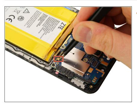
Use tweezers to remove the antenna.
