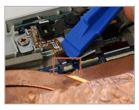
Remove the connector immediately to the left of the front webcam's connector. Use a plastic opening tool to gently lift the connector up and out.
