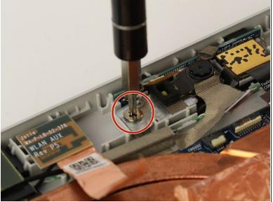
• Use a Phillips screwdriver to remove the Phillips M2.0x2.0 screw to the left of the webcam. Turn the screwdriver counterclockwise to remove the screw.
