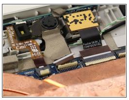
Remove the wire connector to the front webcam using a plastic opening tool. Hook the tool underneath the connector and pull up and back.
