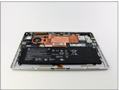
Remove the screen by gently lifting it off of the device.
