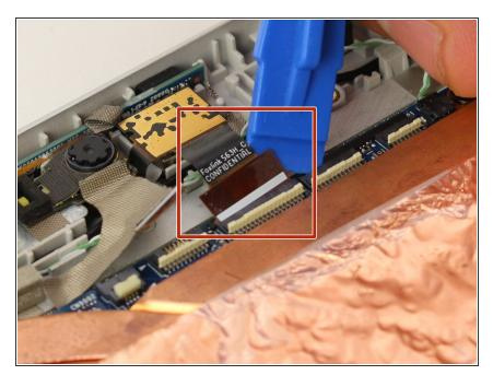
Remove the connector immediately to the right of the front webcam's connector. Use a plastic opening tool to gently lift the connector up and out.
