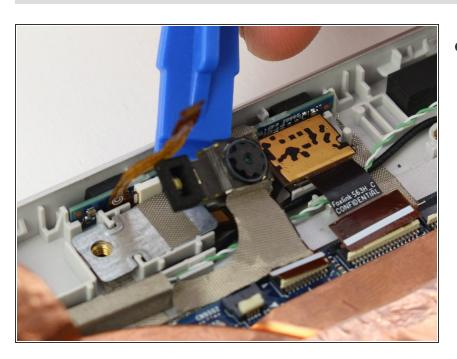
Remove the webcam using a plastic opening tool to lift it up and off.
