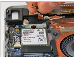
• Detach the two wire connections on the upper right of the wi-fi card by hand.
