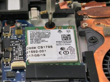
• Use a Phillips 2mm screwdriver to remove the single M2 2.0x2.0 screw holding the wi-fi card in place. Turn the screwdriver counterclockwise to remove the screw.
