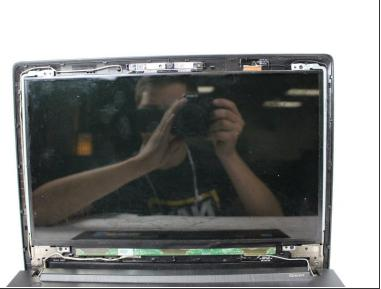
Carefully unsnap the front plastic piece to expose the frame of the screen.
