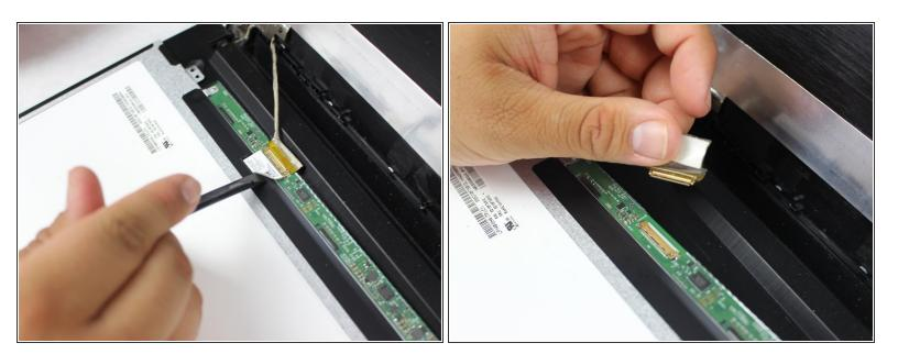
Slowly remove the sticker connected to the rear of the screen using a spudger.
