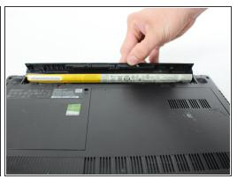
Once both switches are pulled, the battery should pop out.
