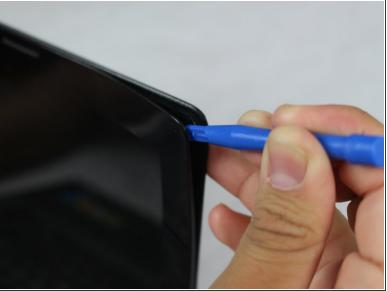
Use the plastic opening tool to pry the plastic away from the screen.
