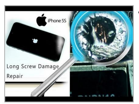
In this guide you will learn about problem with bootloop in iPhone 5s caused by the wrong long screw which destroy the connection path.
