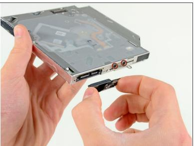
Pull the optical drive cable out of the optical drive.
