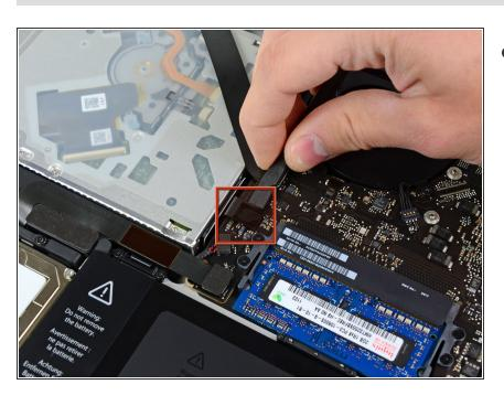
Use the flat end of a spudger to pry the optical drive connector up from its socket on the logic board.
