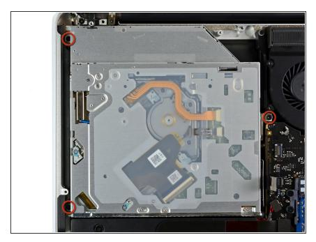
Remove the three 3.5 mm T6 Torx screws securing the optical drive to the upper case.
