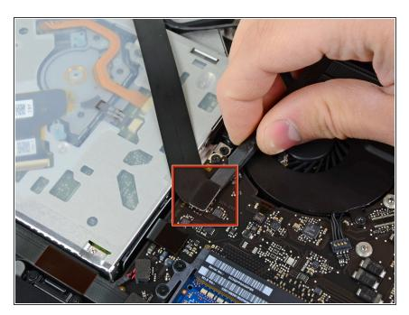
Use the flat end of a spudger to pry the AirPort/Bluetooth connector up from its socket on the logic board.
