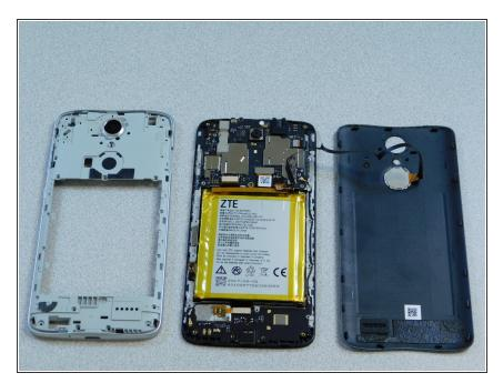
You have reached the Fingerprint Scanner, the device Battery, and Front Facing Camera.
