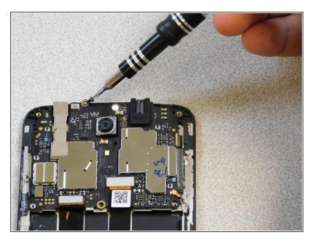
Once you have the power connectors disconnected from the top chipset, use a Phillips screwdriver to remove the final screw located at the very top of the chipset (as shown in image).
