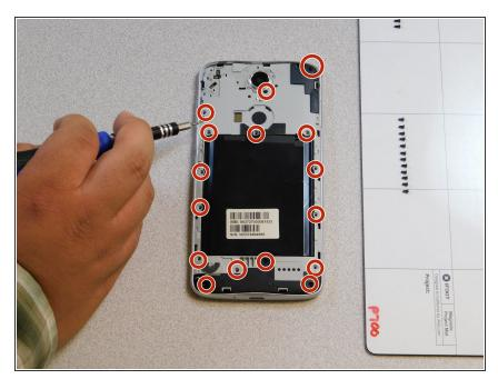
Once opened, Locate and remove all exposed screws using a Phillips-Head screwdriver and set them aside.
