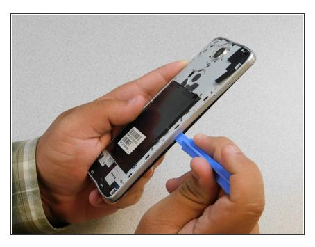
To remove the inner white panel/cover, use a plastic opening tool to loosen from each side.
