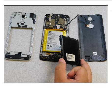
Then, simple lift to remove the metal battery cover.
