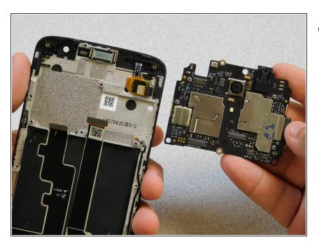
Then, simply lift chipset from top and detach from the device frame.
