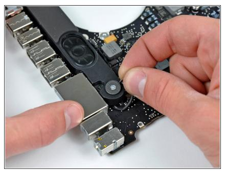
(i) Lift the microphone out of its recess in the left speaker housing.
