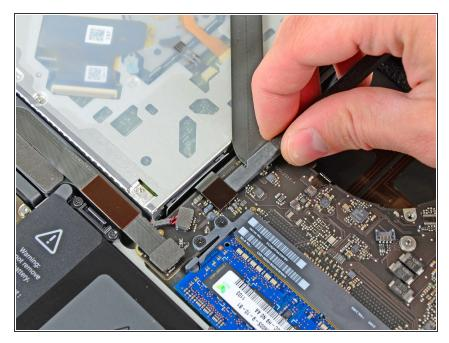
• Use the flat end of a spudger to lift the optical drive connector out of its socket on the logic board.
