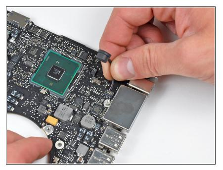
Carefully pull the microphone cables upward to lift the microphone connector out of its socket on the logic board.
