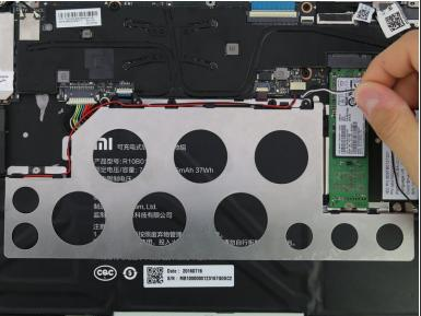
Detach the white and black speaker wires by pulling them from the small black tabs along the perimeter of the metal bracket.
