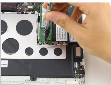
Remove the 1.5mm screw using the JIS #00 screwdriver.
