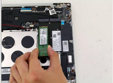
Lift the SSD up from the device and gently pull the SSD from the laptop.
