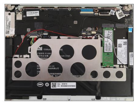
Detach the red wire from the tabs on the perimeter of the metal bracket.
