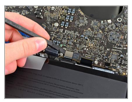
Use the flat end of a spudger to pry the trackpad connector up and out of its socket on the logic board.
