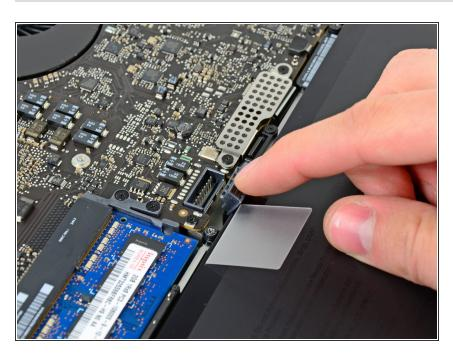
Bend the battery cable slightly away from its socket on the logic board so it does not accidentally connect itself while you work.
