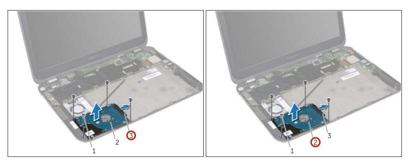
• Connect the hard-drive cable connector to the hard-drive assembly.
