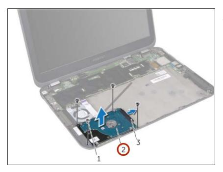
• Lift the hard-drive assembly away from the computer base.
