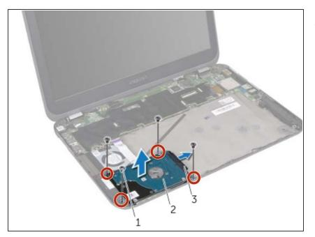
Align the screw holes on the harddrive assembly with the screw holes on the computer base.
