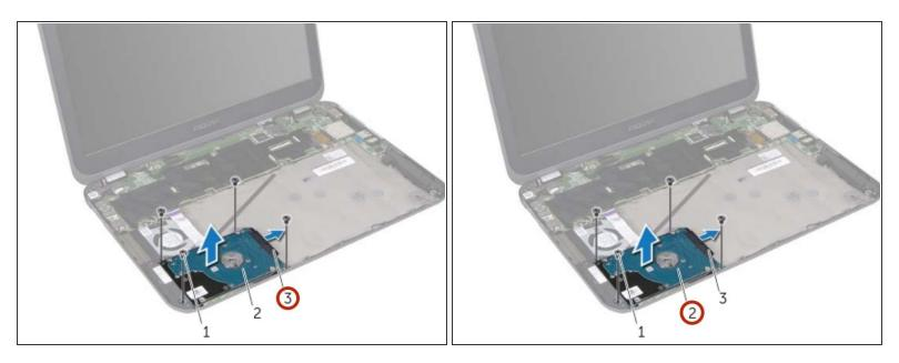
Disconnect the hard-drive cable connector from the hard-drive assembly.
