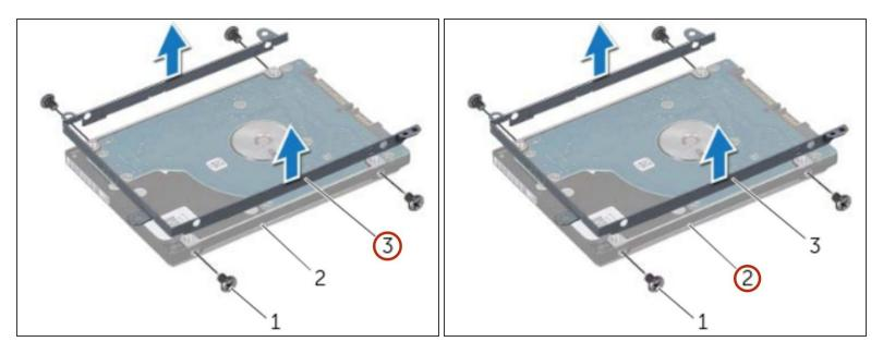
• Lift the hard-drive bracket off the hard drive.
