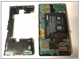
Use the flat end of a spudger to pry the battery cover from the phone's frame.
