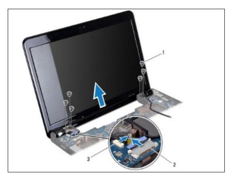
Make note of the cable routing and carefully dislodge the Mini-Card antenna cables from the routing guides.
