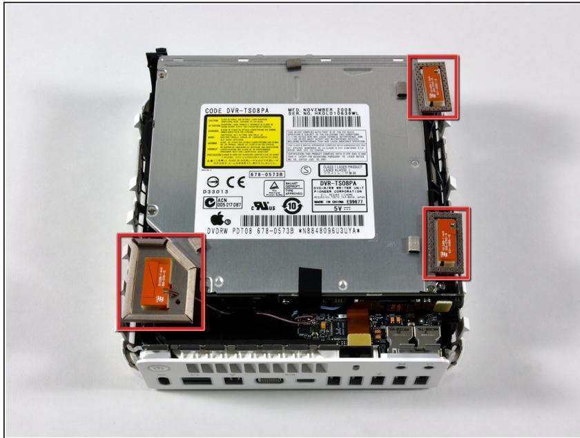
**!** In the next few steps you will be removing the AirPort and Bluetooth antennas (shown in red) from the internal frame. Be very careful, as breaking the brackets will require replacing the internal frame.
