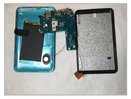
Pick up the motherboard and carefully place adjacent to the battery.
