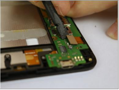
Use the flat end of a spudger to disconnect the ribbon cable.
