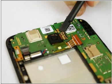
Using the flat end of the spudger, disconnect the camera from the motherboard.
