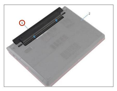
Insert the NEW battery at an angle into the battery bay and align the tabs on the battery with the slots on the battery bay.
