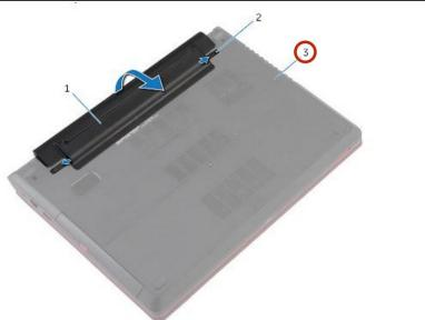
Using your fingertips, lift the battery at an angle and remove the battery off the computer base.
