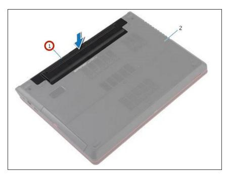
Press the battery down until it snaps into place.
