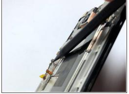
• Use the plastic spudger to loosen the metal prongs that hold the button assembly onto the phone.
