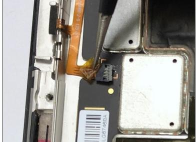
Peel back the orange adhesive covering the ZIF connector.
