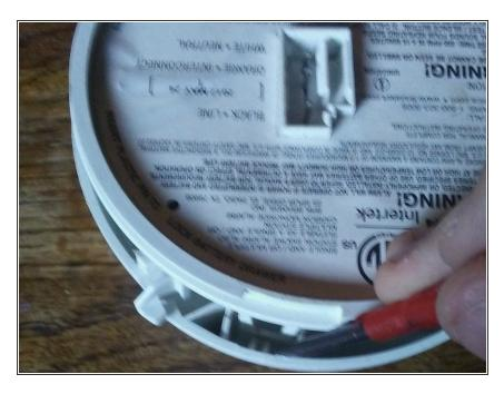
You're going to want to get a flat head screwdriver and pry open the clip on the inside to get to the inner part of the alarm.
