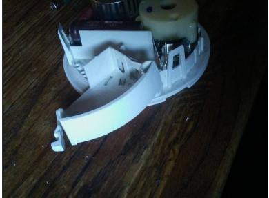
Now what you should do is pop a small screwdriver into the rivet hole to unlock the battery holder.
