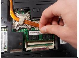
• Pull the metal tabs and lift the first RAM stick out of the socket.
